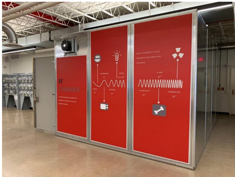
Figure 7: Smart City Lab Radio Frequency Isolation Chamber
